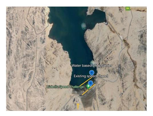
Detailed map of the upper lagoon area with the existing excavated speed channel which is dominantly utilized by the windsurfing athletes. Additionally, the proposed new water-based speed facility in the shallows of the lagoon for the kite surfing athletes. The yellow arrow indicates prevailing wind direction.
