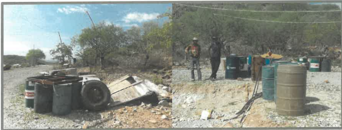
Figure 13: Hydrocarbons that need to be stored in a lockable bunded storeroom (HEEC, 2023)
