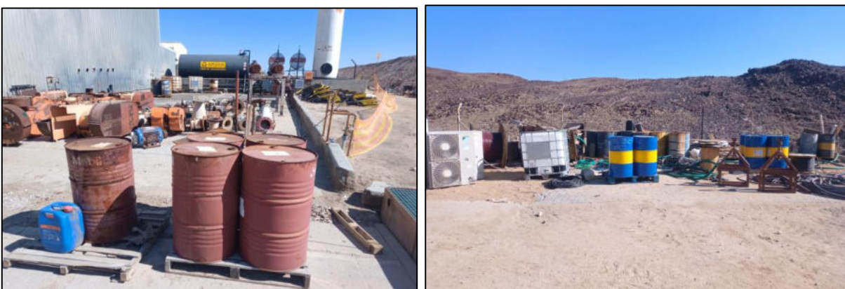
Photos 4 and 5: Hydrocarbon storage – outside bunded areas
