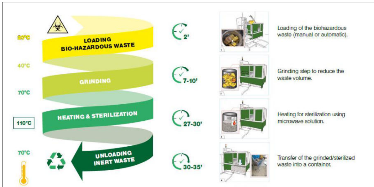
Figure 3-1: Graphic representation of the treatment process of the STERILWAVE apparatus
