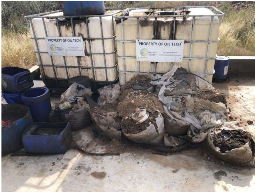
FIGURE 4: STORAGE OF USED OIL, EMPTY CONTAINERS AND HYDROCARBON-CONTAMINATED WASTE IN A SEALED, BUNDED AREA
