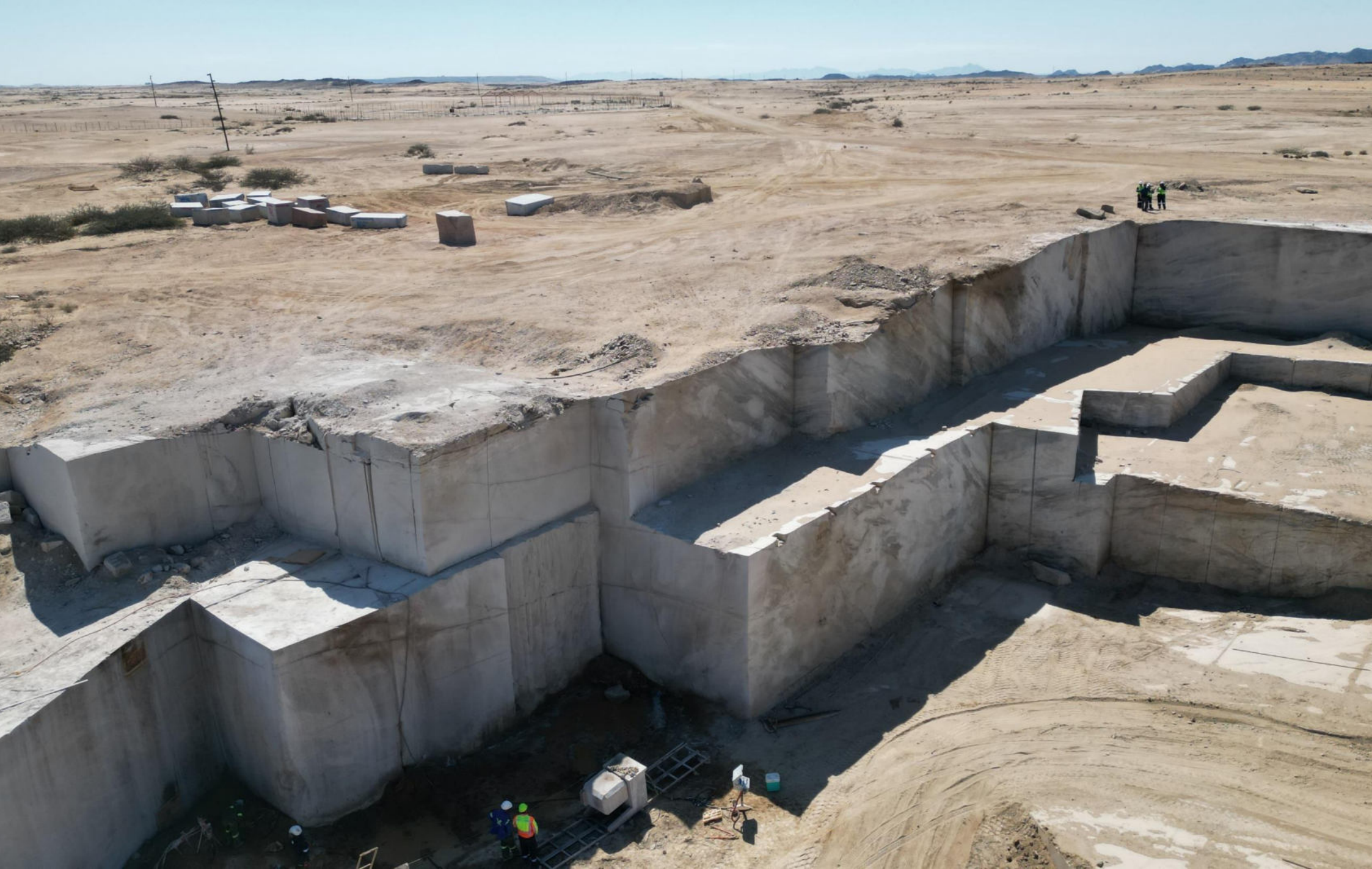
Plate 2.7: Extraction \ mining face of the rectangular blocks, stockpiled and sorted before being transported to the plant for final processing.
