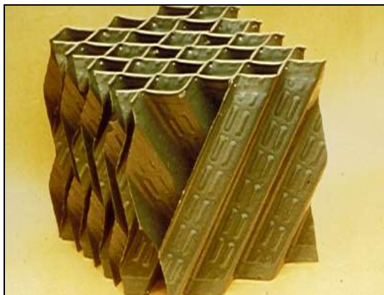
Figure 9a): Packing in trickling filter.
