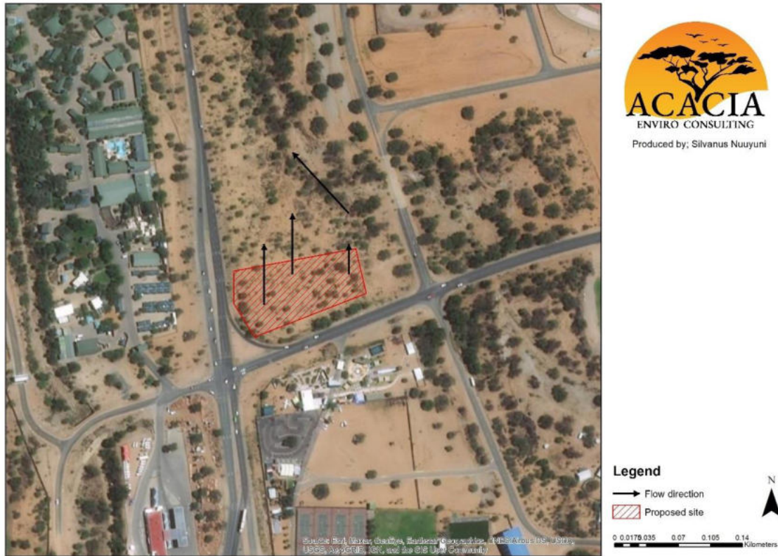
Figure 6: Surface water flow direction
