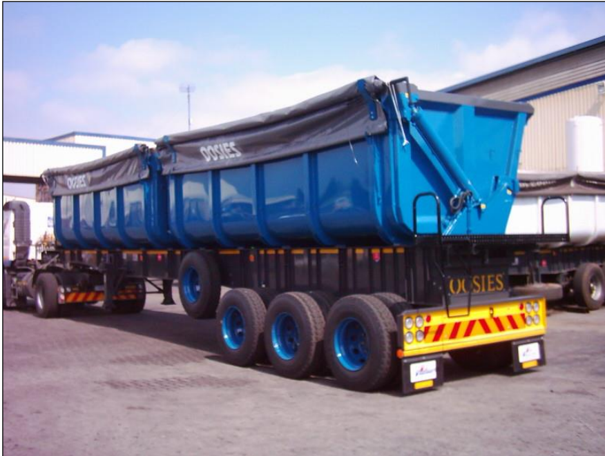
Plate 1: Example of side tipper unit.
