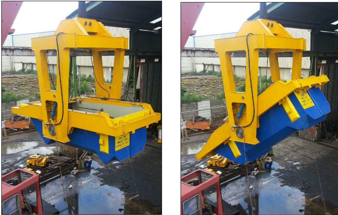
Plate 7: Illustration of the 90 degree tipping containers to be used for the ship loading.
