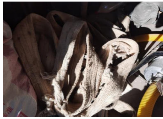
Damaged slings in use
