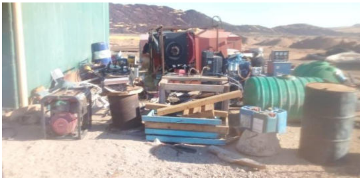
General field equipment behind the container equipment warehouse. Note that generators and drilling fluid containers are placed on the floor directly
