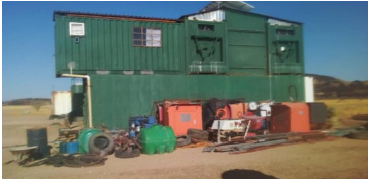
General field equipment behind the container equipment warehouse. Note that generators and drilling fluid containers are placed on the floor
