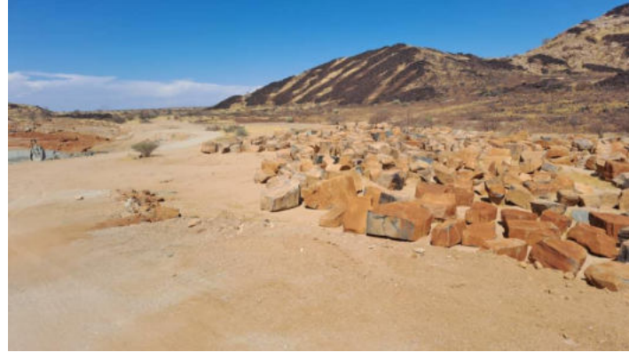
View of loose dolerite boulders stripped off from area where the eastern test quarry has been developed
