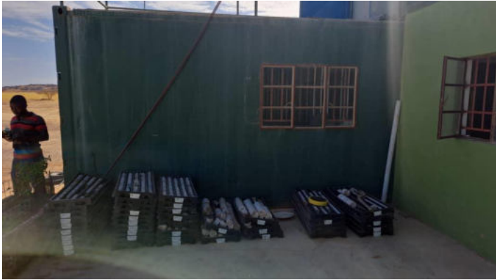
Diamond drill core storage area at the exploration camp. Core largely retrieved from drill holes drilled to facilitate wire saw cutting
