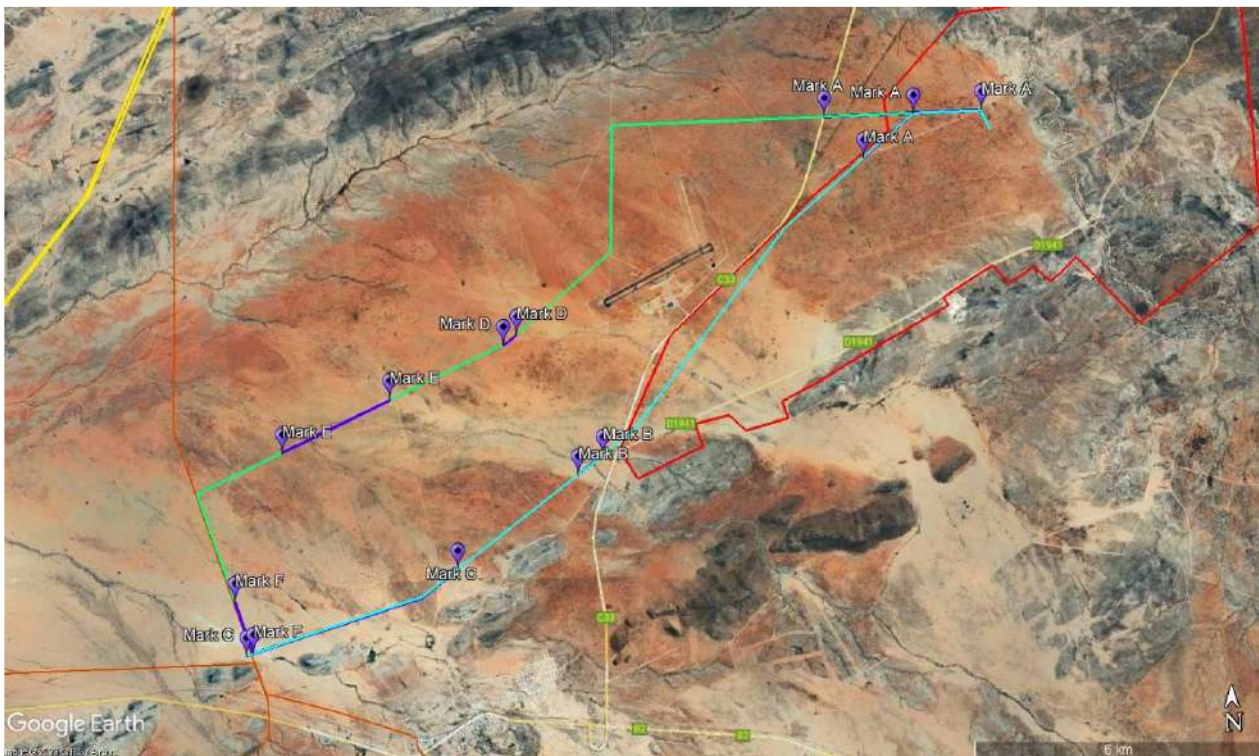
Figure 13 - Recommended sections of powerline to be marked for the proposed 66kV powerline for the two routes
