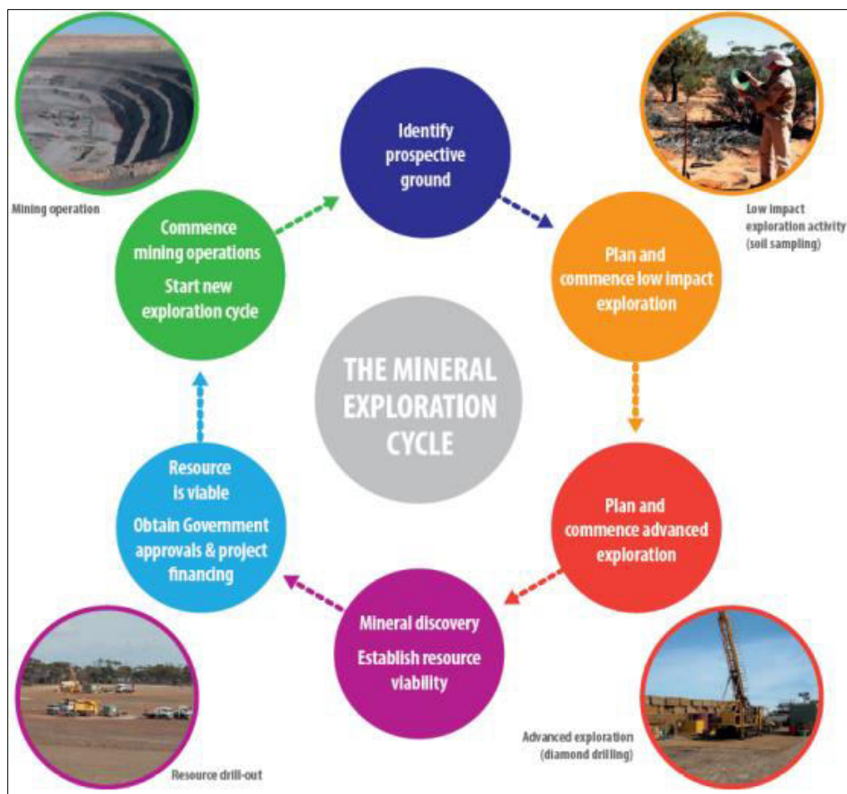
Figure 2: The mineral exploration cycle (Source: Dept. Energy & Mining – Government of South Australia, 2021)
