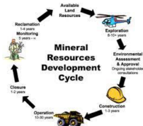
Figure 3: Diagram of the major steps involved in a mining process (Socratic, 2016)
