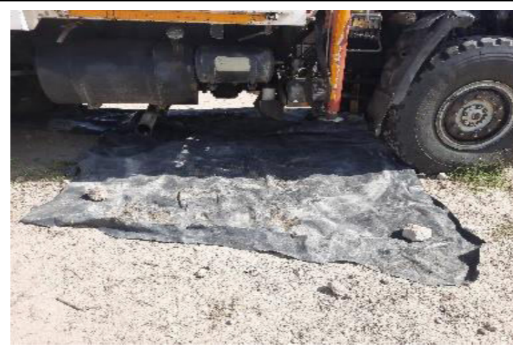
Insufficient and ineffective bunded area
