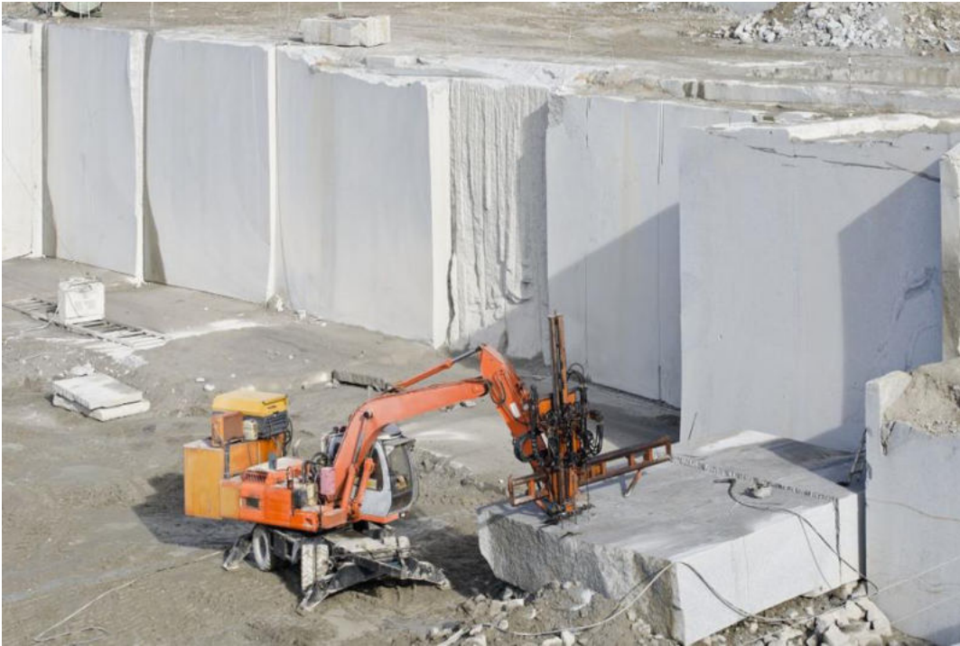
FIGURE 5 - WHITE MARBLE QUARRY CUTTING OPERATIONS
