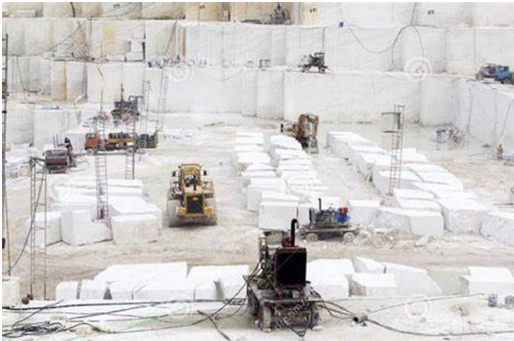
FIGURE 7 – TYPICAL ON-SITE BLOCK SORTING AND STOCK PILING
