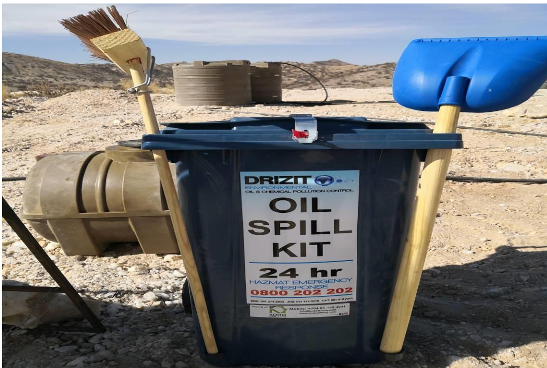
Figure 6 – Photo (DLE)- Oil spillage containment kit at one of the drill sites over a historical coarse mine dump
