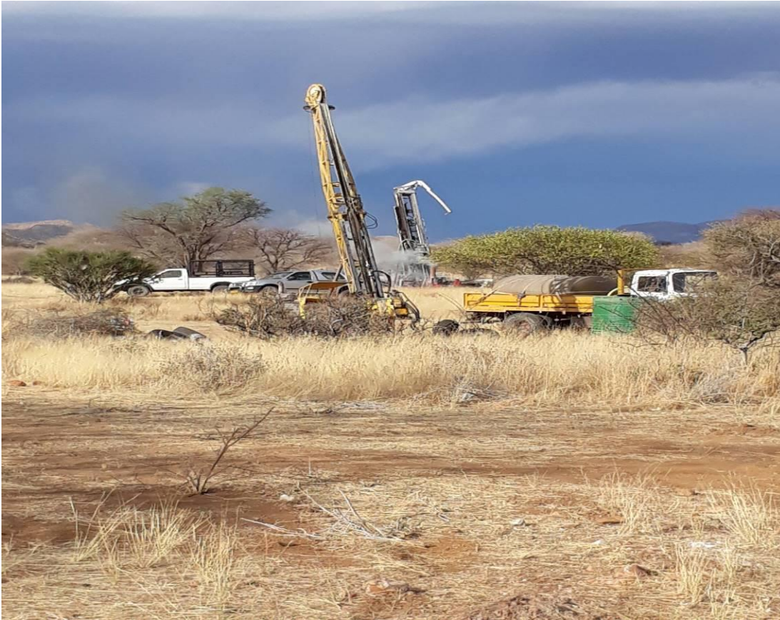
Figure 5 - Photo (DLE) - One diamond Rig & RC rig drilling adjacent to each other at Rubicon
