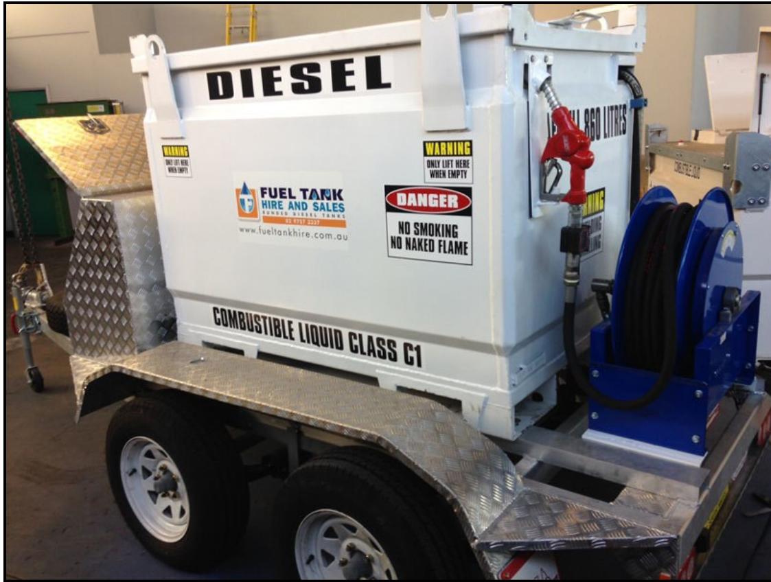
Figure 9: Self bunded fuel tank on trailer for storage and dispensing of diesel
