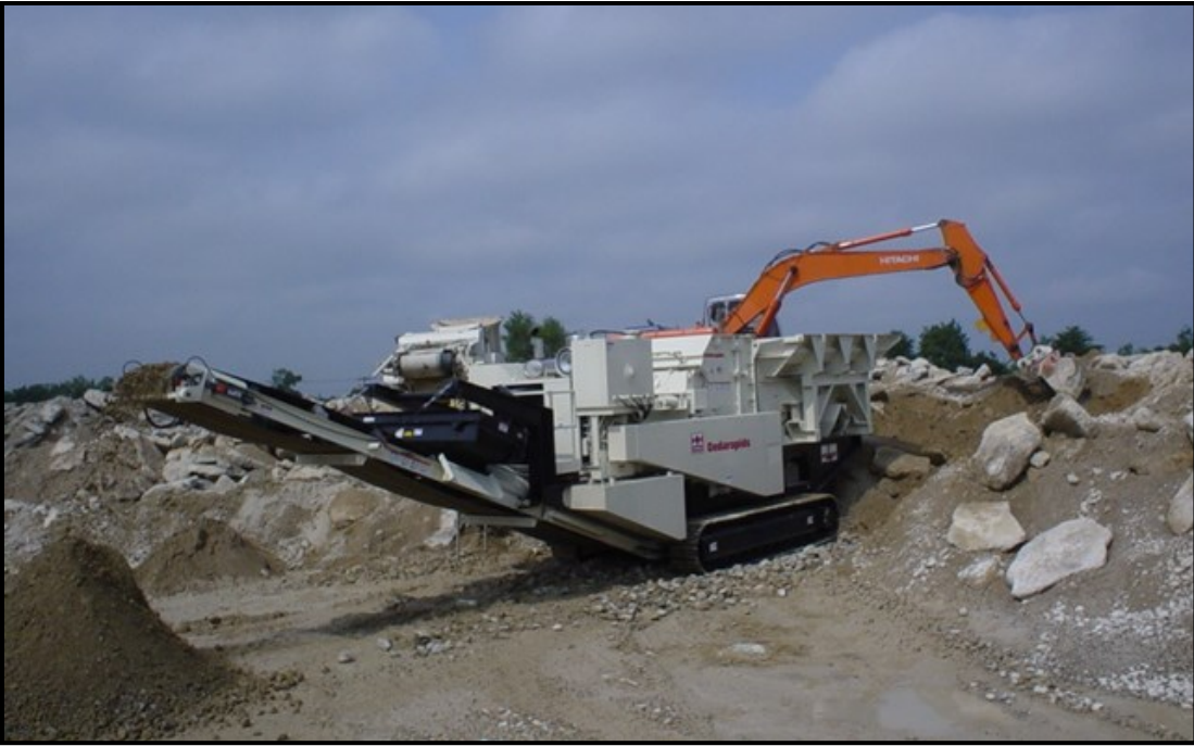
Figure 5: Example of excavator loading from dump into a mobile crusher
