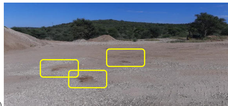
Figure 6: Pictures showing: a) the drum for the collection and storage of the waste oil; and b) areas contaminated with hydrocarbons (Source: L. Maartens, 08 March 2023).
