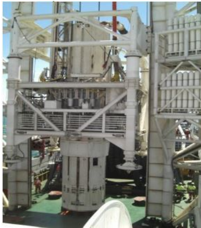
Figure 06. The 2.5m diameter drill bit within the drill frame structure.
