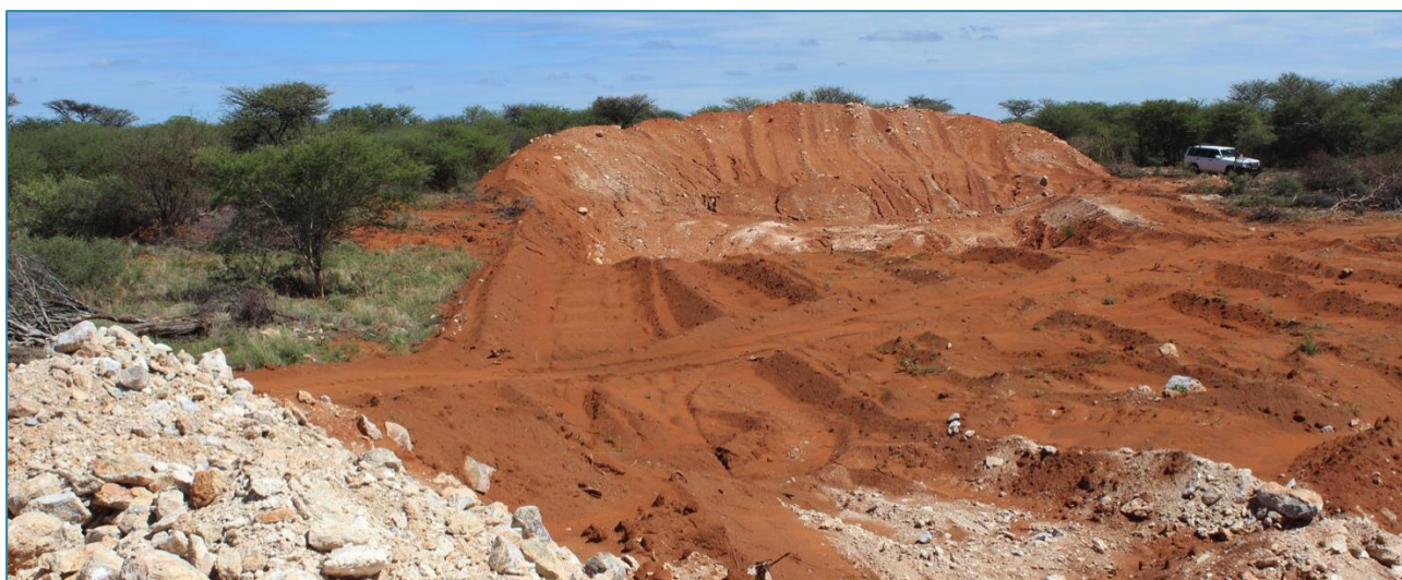
Fig 8: Shows the stockpile of overnuden consisting of both the soft topsoils and the rock materials stored separately in favor of the rehabilitation process once mining is completed.
