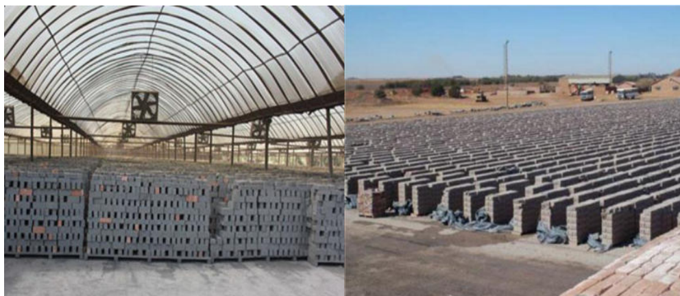
Figure 9: Bricks being dried mechanically (L) & Natural open air drying (R)
