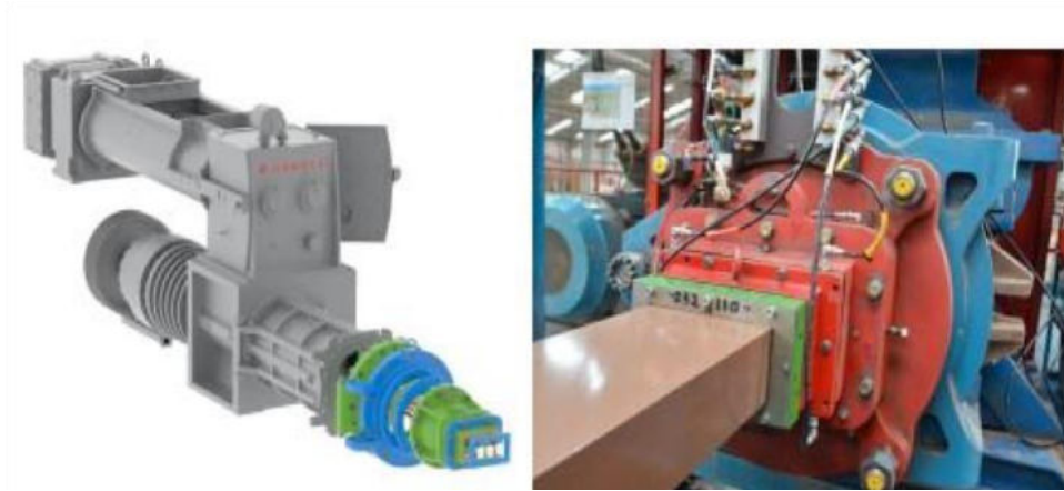
Figure 8: The Extruder Machine (L) & A column of clay being extruded (R)
