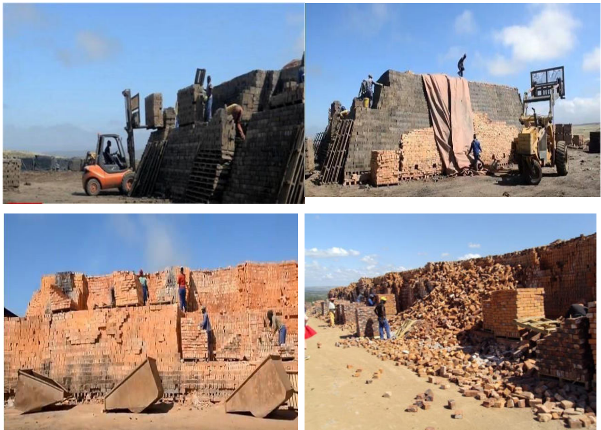
Figure 10: Dried brick being packed on a clamp for firing (top left) & A packed clamp being covered with tarpaulin to protect bricks against rain (top right)
