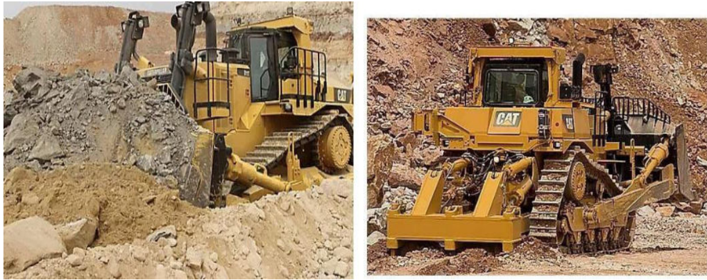
Figure 7: Bulldozer dozing materials (Left) & Bulldozer ripping (Right)
