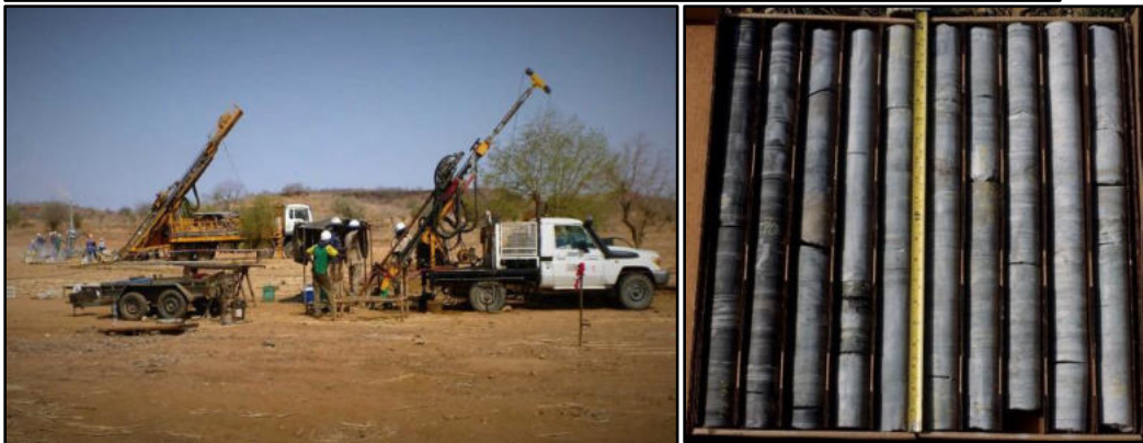
Fig. 9. RC and diamond drilling rigs at work also shown is drill core (activities are very localized with limited footprint).
