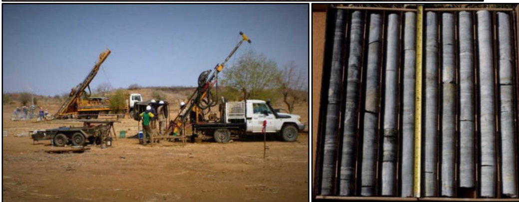
Fig. 14. RC and diamond drilling rigs at work also shown is drill core (activities are very localized with limited footprint).
