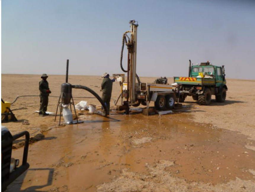
Figure 2 - RAB drilling at Koppies
