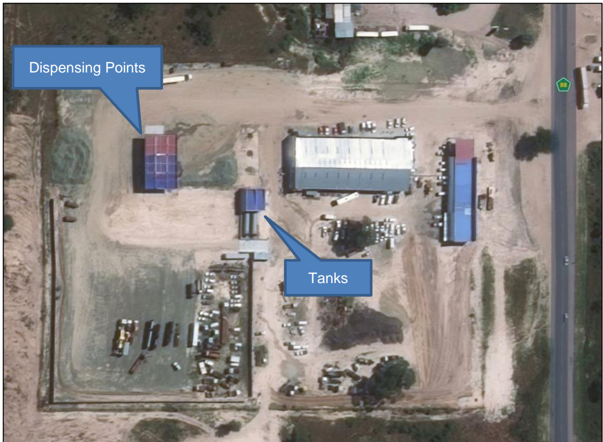
Figure 6: Position of dispensing point and tanks
